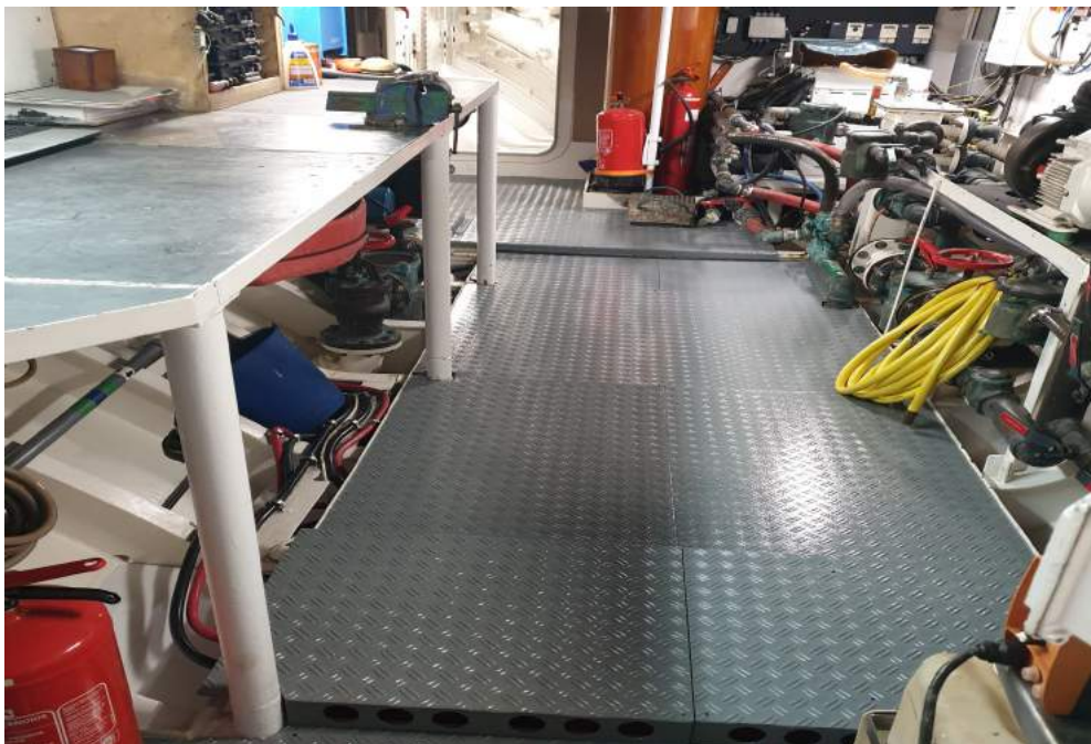
Engine and pump room floor boards repainted
